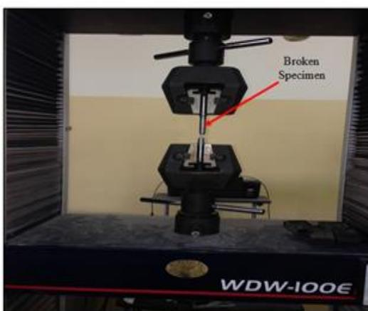
Fig. 4:Tensile testing machine
