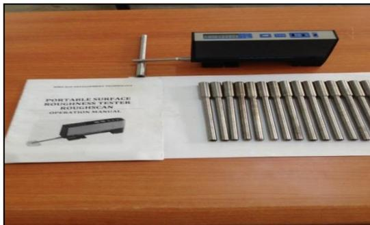
Fig. 5: Portable Surface Roughness Tester
